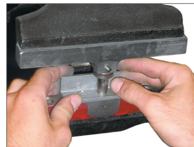
Bench vise used vertically as a press.
