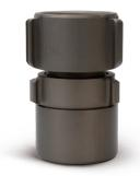
Typical coupling supplied with Municipal and Industrial Hose. Twice as strong as brass and only one-third the weight. Hard-coated for extra wear resistance and helps prevent damage to swivel and threads. Three lugs on both male and female swivel. Expansion ring type.
