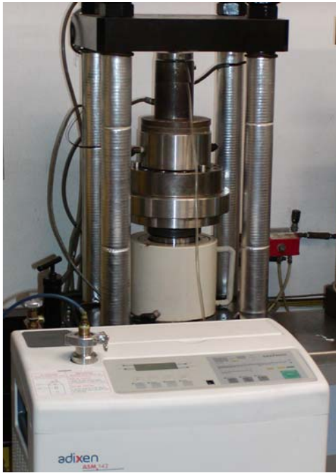
FIGURE 3 – TEST RIG, HYDRAULIC PRESS AND He MASS SPECTROMETER
