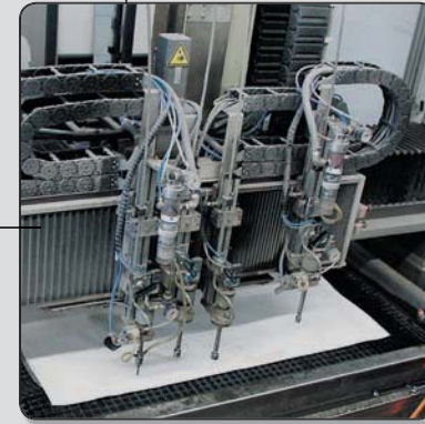
Computer Controlled Gasket Cutting
