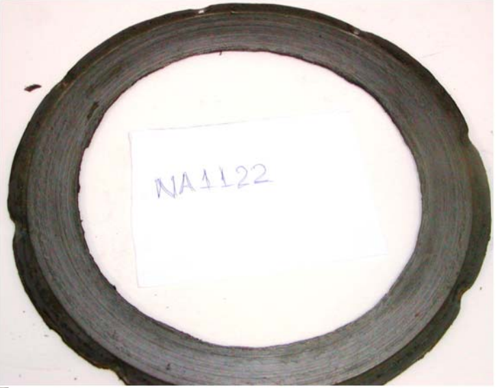
Figure 6: Teadit NA1122 after disassembled.
