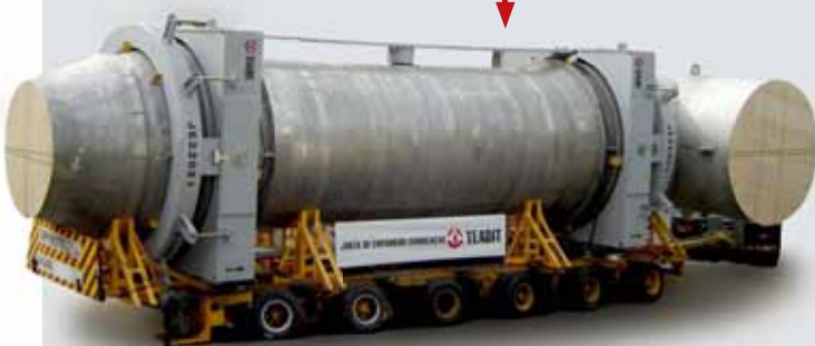
Gimbal Universal Hot-wall Expansion Joint - ID 120 in / 50 ton
