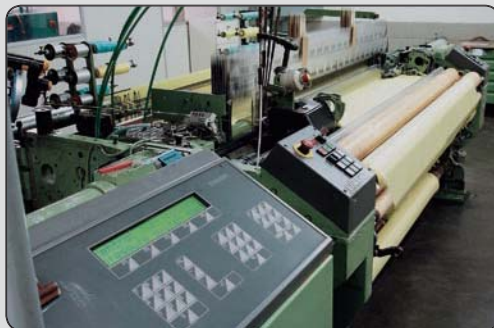
Rapier Loom with Load Cell Warp Control
