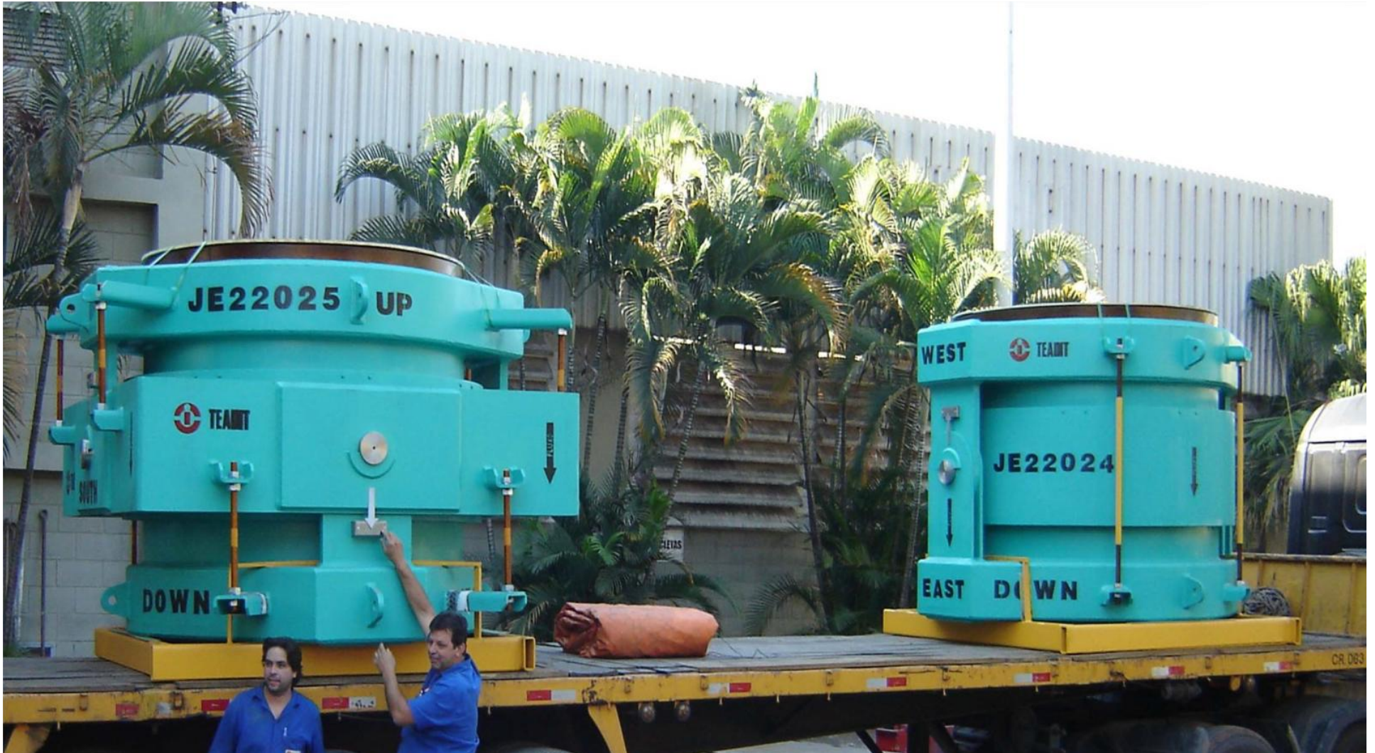
Gimbal Cold-Wall ID: 64 in L: 80 in W: 14 ton
