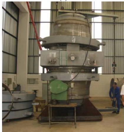
Fig. 4. Expansion joint in the test position (unit in mm). (a) Schematic draw of the test device and (b) Test device build of.
