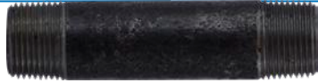
3/4" DIAMETER DIAMETER BLACK EXTRA HEAVY XXS SEAMLESS Wall Thickness 0.308 - Grade B - Test Pressure 1000 PSI - Thread Length 0.79
