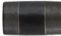
2" DIAMETER DIAMETER BLACK EXTRA HEAVY XXS SEAMLESS Wall Thickness 0.436 - Grade B - Test Pressure 2500 PSI - Thread Length 1.06
