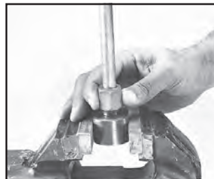
Step 5 – Manually screw nut onto Ferulset Tool or fitting body until finger tight.
