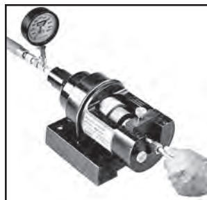
Fig. R29 — Flaring with Hydra-Tool
