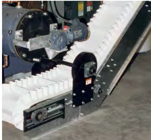
Durowall lightweight belts are popular for operating in confined areas, particularly when products need to be quickly elevated
