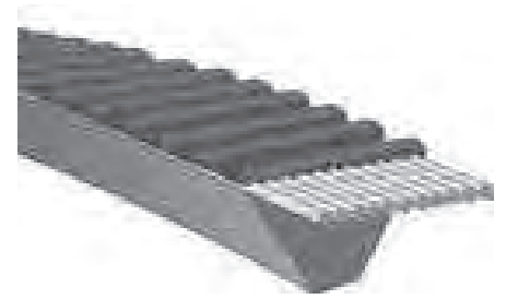
Part Number: 5M 710 5M 5mm (3/16 in.) top width 710 710mm (27.95 in.) outside length
